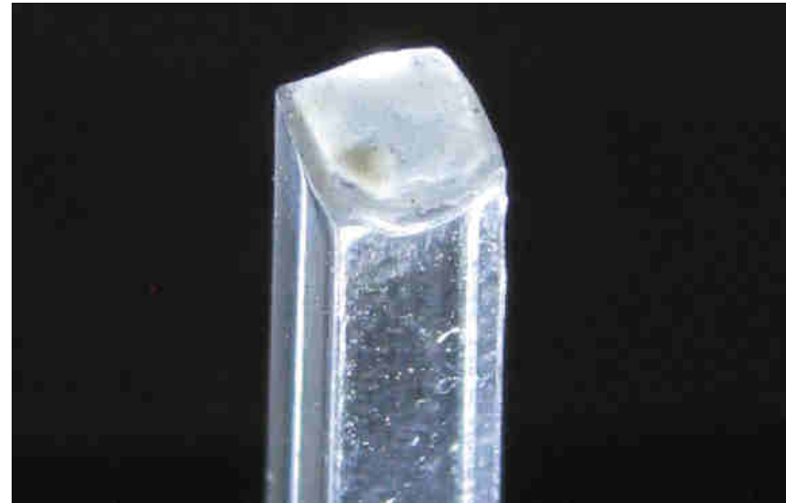
PMMA light guide irreversibly damaged by moderate LED radiation.
